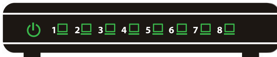
Figure 5.8: A network hub with 8 ports
